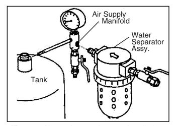
**Figure 7.** Air supply control system installation.
